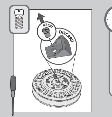
Remove the shipping blocks from the motor. Save the five screws. They will be needed for blade iron installation.
